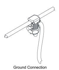
Provides both a mechanical and bonded electrical connection when joining tray sections to one another. Only one CB-10 required per connection.
