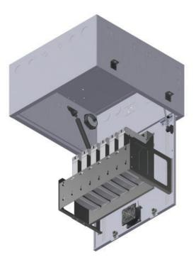
**Applications:** This fully assembled ceiling mount enclosure with Integrated Power Supply installs in 2' x 2', 2' x 4' and 2' x 6' drop ceilings. 6 RU of standard 19" passive rack mountable space and is fitted with a horizontal cable slack manager. Door has a capacity of over 50 pounds and can be customized to user specifications to accept other component structures.
