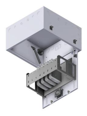
**Applications:** This fully assembled ceiling mount enclosure installs in 2' x 2', 2' x 4' and 2' x 6' drop ceilings. 6 RU of standard 19" passive rack mountable space and is fitted with a horizontal cable slack manager. Door has a capacity of over 50 pounds and can be customized to user specifications to accept other component structures.
