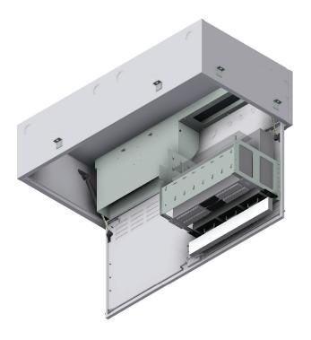
Applications: Secure consolidation point for distributed network equipment. Lessens the heat load and density in the Telecom Room. Flush mounted, white enclosure installs into a standard 2' x 2' grid ceiling. Architecturally pleasing metal bezel with hinged door complete with vented louvers. Powder coated for seamless integration into any office environment.
