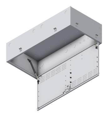
Applications: This fully assembled extra large ceiling mount enclosure installs in 2' ceiling grid, measures 2' x 4'. This particular model can be mounted with 12 RU of standard 19" passive rack mountable space and horizontal cable slack managers. Lockable secure door has a capacity of over 75 pounds and can be customized to user specifications to accept other component structures. Vented cover opens safely with two built-in pneumatic cylinders. Single lockable handle.
