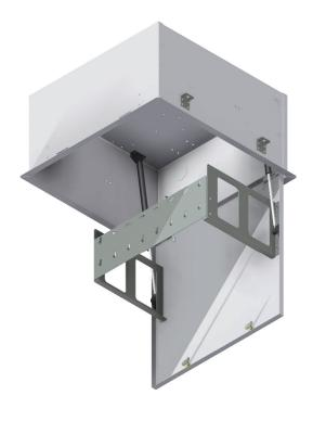
Applications: This fully assembled ceiling mount enclosure installs in 2' x 2', 2' x 4' and 2' x 6' drop ceilings. This particular model has 6 RU of standard 19" passive rack mountable space and is fitted with a horizontal cable slack manager. Lockable secure door has a capacity of over 50 pounds and can be customized to user specifications to accept other component structures. Cover opens safely with two built-in pneumatic cylinders.
