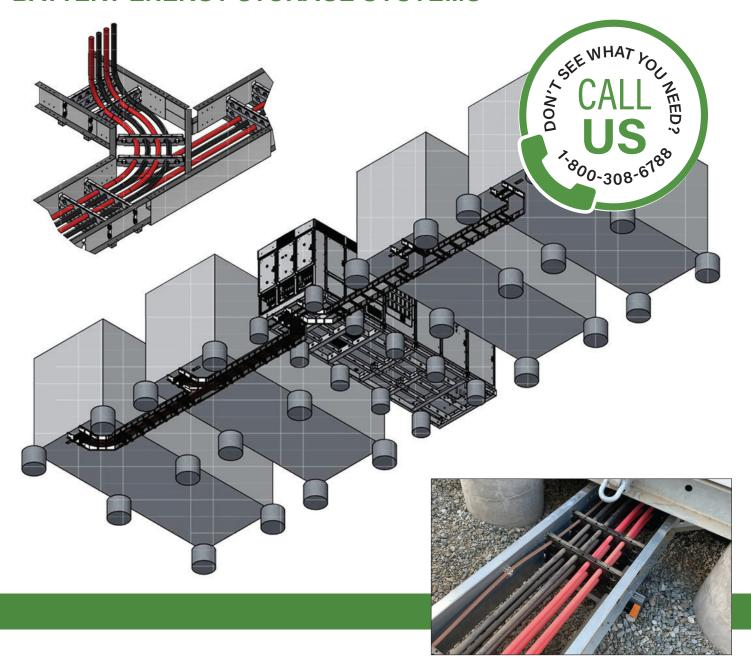
Solar Snake Max XL™ For Battery Energy Storage Systems (BESS) Cable Management For Interconnecting the Batteries to the Inverters, Utility or Solar Farm
