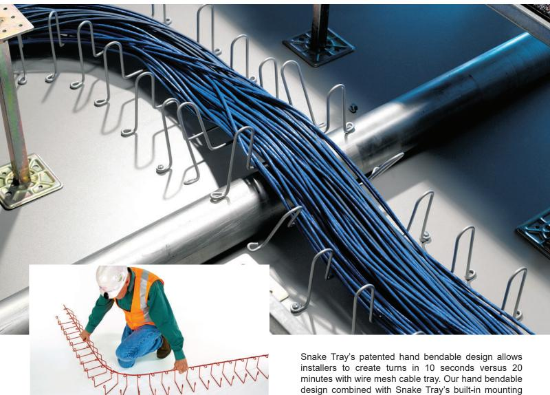
The 101 series Snake Tray is designed for installation below a raised floor and as a riser along vertical surfaces. Available in several sizes, the 101 series tray can accommodate up to 84 square inches of cable path or 860 data cables. Support legs and mounting rings are pre-formed into the tray and require no additional brackets to install. Custom sizes available.
