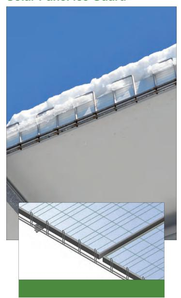
Snake Tray's Solar Panel Ice Guard helps to aid in the prevention of ice and snow from falling off the surface of the solar panels. The system easily mounts to the frame of any solar panel and is designed to hold back frozen material up to the top edge of the guard, helping to protect pedestrians and vehicles from the dangers of falling ice.
