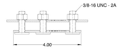
The CM 801-SP provides a mechanical connection and an electrical bond when joining the Mega Snake Tray sections to one another.
