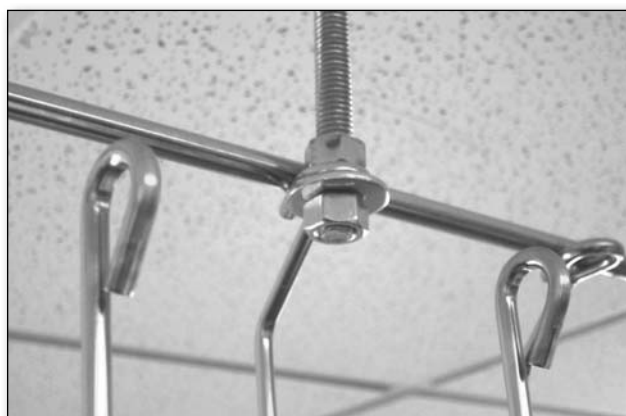
Figure 3 - Suspending Snake Tray from threaded rod using the "Snake Eyes"
